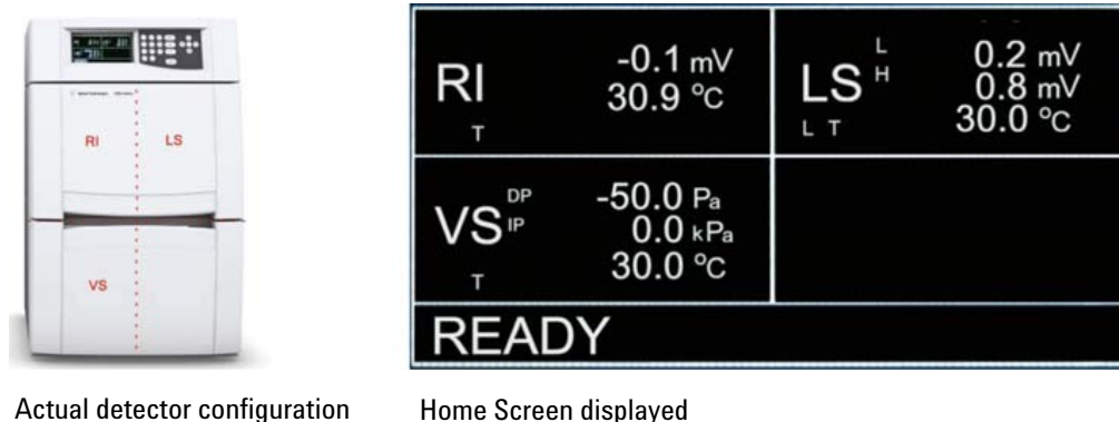
Figure 11 MDS with RI, LS and Viscometer (VS) Detectors
