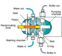
Rugged, single-piston design saves time and seal replacement costs.
