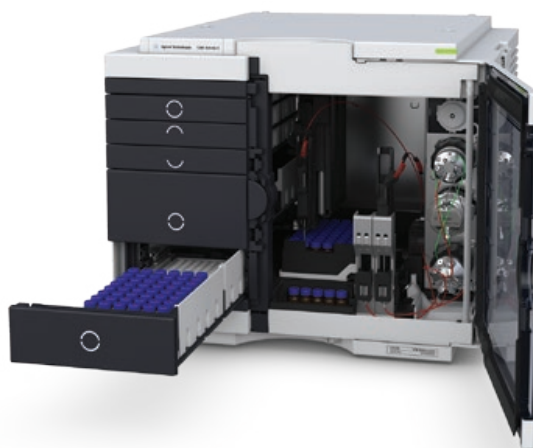
The 1290 Infinity II Multisampler – fast injection cycles and high capacity within the footprint of a standard Agilent LC stack
