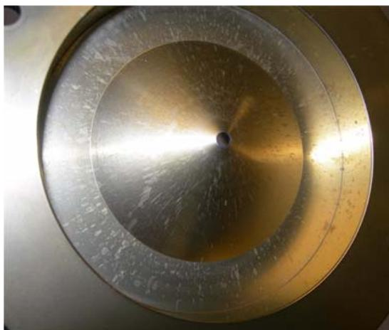
**Figure 19** Sample splatter on skimmer
