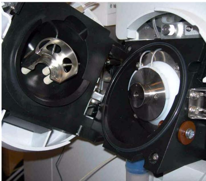
**Figure 6** Opened electrospray spray chamber
