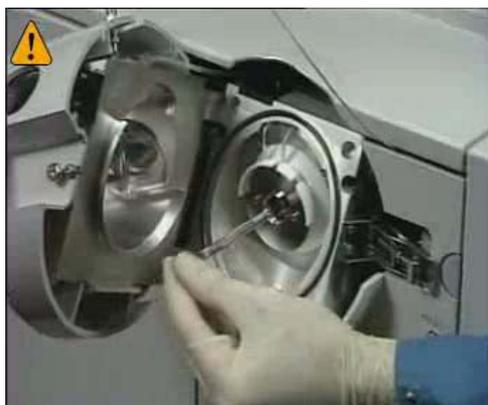
**Figure 56** Reinstalling the capillary
