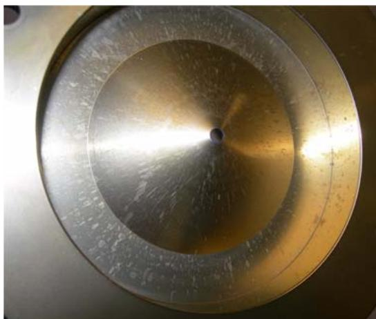
**Figure 57** Sample splatter on skimmer
