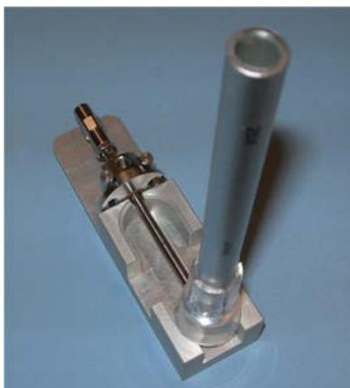
**Figure 11** Electrospray nebulizer needle in needle holder
