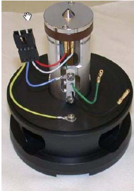
**Figure 69** The re-assembled ion optics assembly
