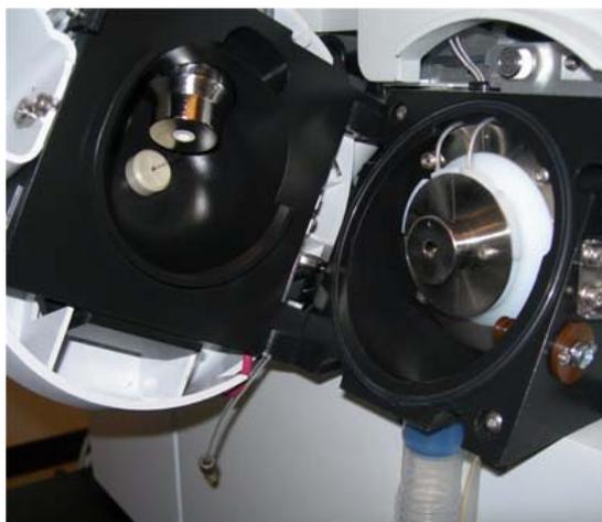
**Figure 34** Opened spray chamber
