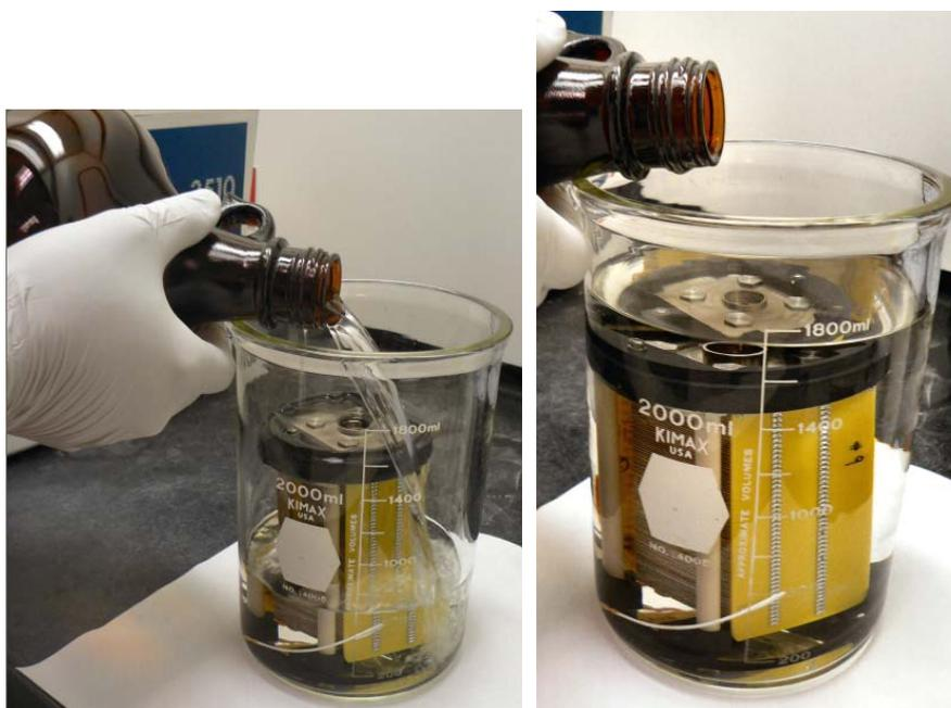
**Figure 74** Pouring isopropanol into the glass beaker.
