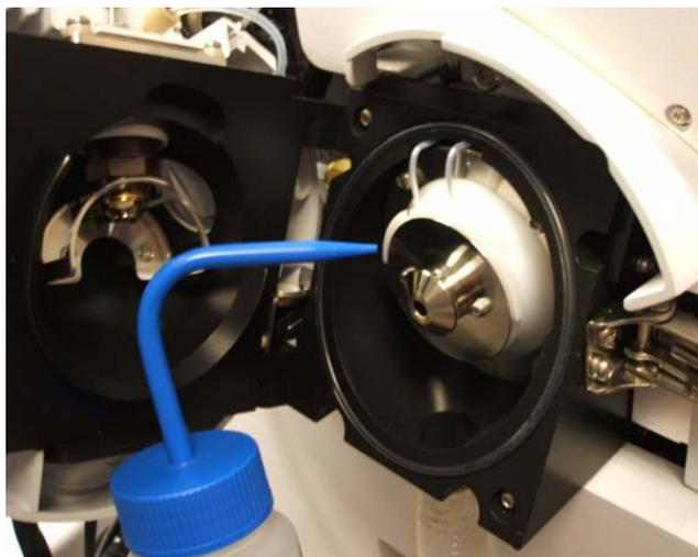
**Figure 9** Rinsing the area around the spray shield
