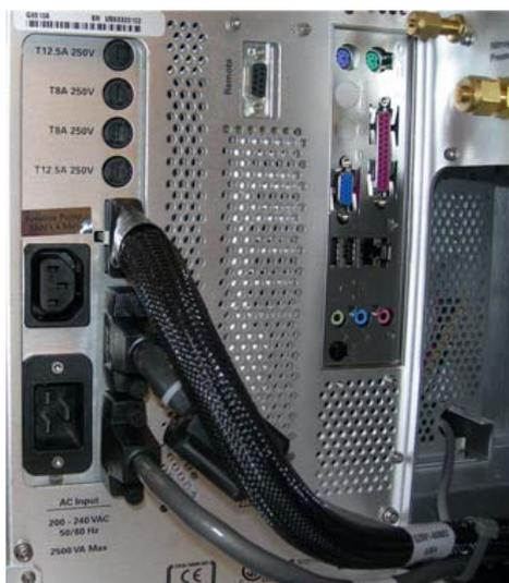
**Figure 78** Disconnect the instrument power cable.
