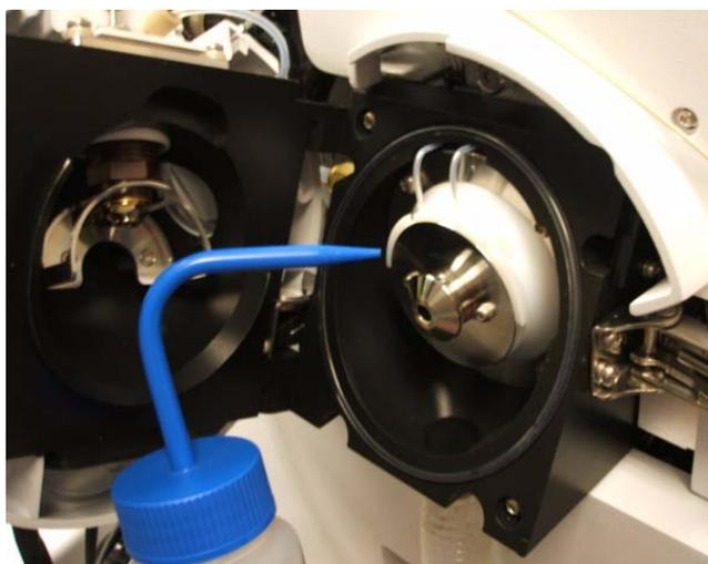
**Figure 24** Rinsing the area around the spray shield
