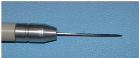
**Figure 44** APCI corona needle after cleaning.
