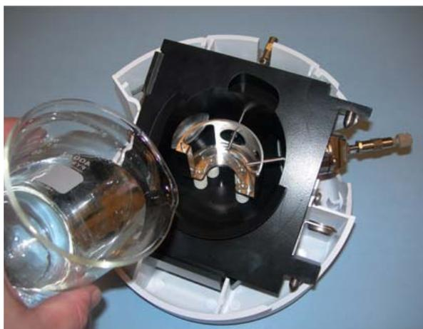
**Figure 7** Filling the spray chamber
