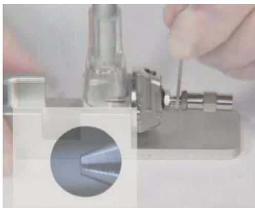
**Figure 41** Adjusting the needle holder
