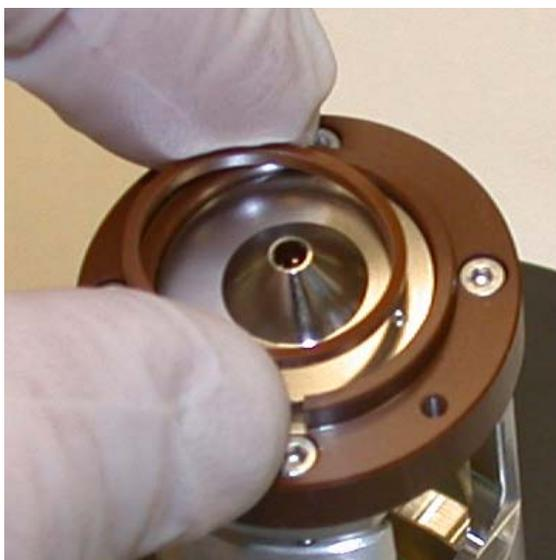
**Figure 66** Spacer insulator
